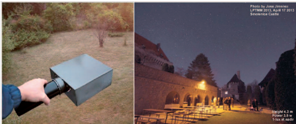
Figure 13 The Canadian Scotobiology Group (CSbG) luminaire has been patented. It is a compact unit with LED light sources powered through an adjustable driver for 110 Vac, 220 Vac or 277 Vac. The thermal design maintains the LED junction temperature to less than 50°C above ambient air temperature at maximum light output, though more typically 20°C for intermediate power settings. The unit was demonstrated at the 2013 Conference on Light Pollution Theory, Modelling and Measurement (photo by Jose Jimenez). The luminaire was mounted at 4.3 m and set for 3.5 W, producing 1 lux at nadir. The main mirror was set for an optional 1.5 m backlight
